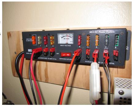
the DC distribution box is individually fused for the correct rating. The extra bits of cable can then be saved and used if the radio is removed from the shack and put back into mobile mode by adding more Power Pole connectors—ergo, no waste and no extra cables have to be purchased.
